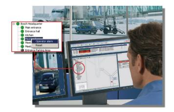
The operator alarm feature allows an operator to trigger an alarm manually from the location tree, for example, if informed by telephone of a dangerous situation. Such manual alarms are processed in the same way as those triggered by a detector: that is, the associated documents are displayed and all steps taken are recorded in the event log.
